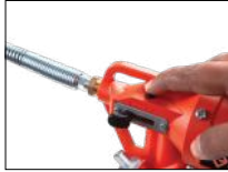
Press button for ONE SHOT OPERATION
