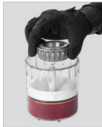
Place bearing on piston Maximum bearing dia. 3-1/2" (90mm)
